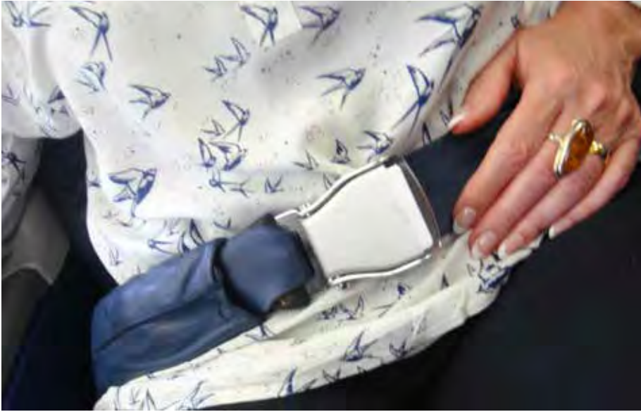
Left: An airbag is contained within the belt, alongside the buckle.
